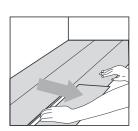
Do not bend connected planks backwards as this will damage it.
